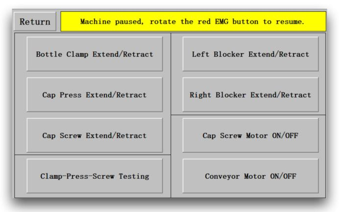
In here, you can manually control all the moving parts on the machine to test whether if it's functioning well or not.
