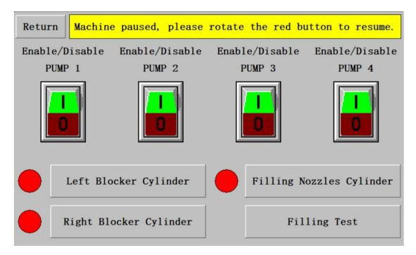
In here, you can manually control the movement of the 3 cylinders, kinda like a debug mode to find out whether if there's any malfunctions, also you can shut the pumps down individually here if you like.
